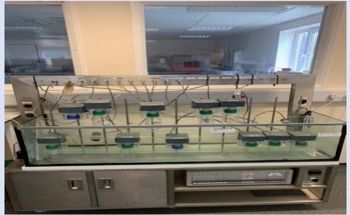
Figure 1 – A respirometer used to measure the rate of oxygen consumed by the microorganisms
